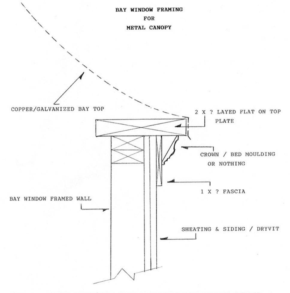
NOTE: TO PREVENT STAINS DOWN FRONT OF BAY WINDOW ALLOW A MINIMUM OF ONE INCH OVERHANG BEYOND CROWN MOULDING.
